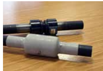
Lokrings coated in Belzona
